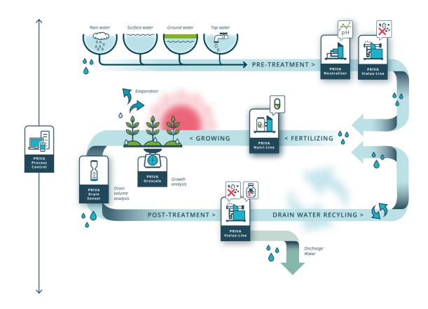
The Priva water management program is an integrated total modular program of measuringand control functions. Priva water management includes controls for pre-treatment of supply water, dosing of nutrients as well as disinfecting of drain water and the preparation for re-use.
